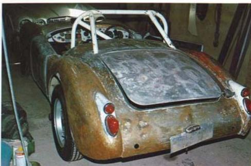
Boot lid rework suffered from previous luggage rack mounting marks and engine bay once hosted a potent 1840 cc motor in place of 1650
